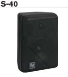
Delivering high performance in an ultra-compact package, the S-40 is ideal for both distributed and near-field applications requiring high-quality sound. The two-way short-throw system is housed in an optimally vented, high-impact polystyrene enclosure that is suited for installation both indoors and out. Lows are handled by a 5.25 inch direct-radiating woofer with a polypropylene cone, while the high-frequency section is a
