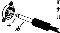
Insert plug into the center of the Speakon-Combo jack. Use only heavy duty speaker cables.
