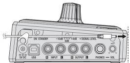
② Turn the tip of the power cord so that it is facing towards you, then turn it back to create a ring as shown in the diagram and insert it into the [5V DC] terminal of this unit.
