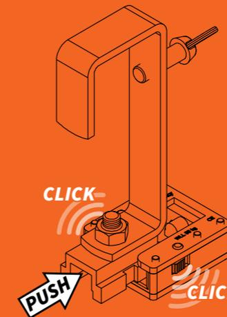
Push the clamp part against the spring block inside the Luminaire part until both locking switches are activated.
