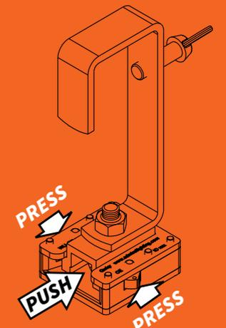
Pull the hook backwards into the housing, press both locks and slide the hook outwards.
