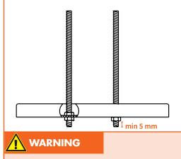
Always tighten the nyloc nut on the bottom of the Truss bracket in such a way that there is 5mm thread visible below each nut. Connecting the U-wire bracket by using M8 nyloc nuts.
