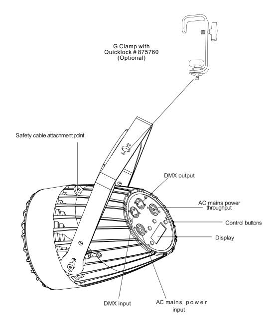
Note: head fan grill in production models is rotated 90° compared to this illustration.
