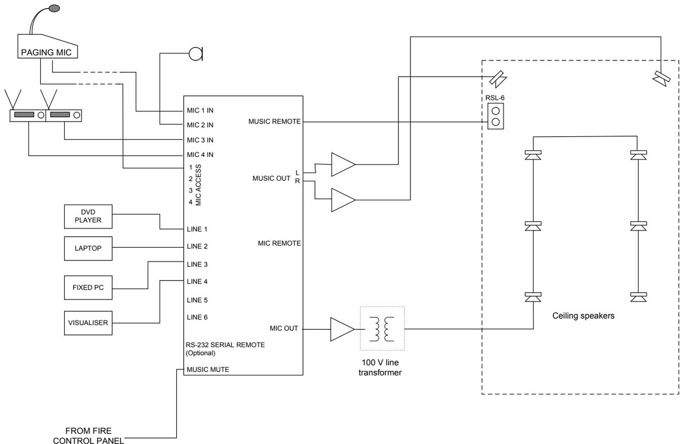
The example shows a CX462 in use in a school classroom. The stereo music output feeds a pair of programme speakers at the front of the room (either side of a display screen), and will receive mainly the programme audio from the various sources but the microphones may be added in as well, as determined by the "Add Mic" control. The music source and volume may be set by means of the local
