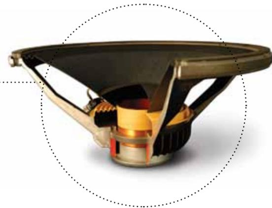
**Bl** Expressed in Tesla meters is a measurement of the motor strength of a speaker. This is created by the product of the magnetic field strength times the length of wire in the field. If you were to take a given mass, that when placed on the cone of a speaker would move the cone downward from its home position, then measure the current in amperes required to move the cone back to home position, you can calculate Bl. The formula is Ma in grams divided the current in amperes.
