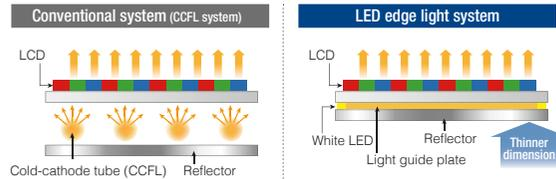
The CCFL system requires the installation of multiple tubes that illuminate in the same way as fluorescent lamps behind the LCD panel. Thus, the display unit becomes thick.
