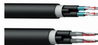
The CSB124 & CSB224 are stereo balanced signal cables featuring a Flamoflex™ outer jacket compliant to the IEC 60332-1 standard regarding fire and flammability resistance in public installations. The Flamoflex™ material is specifically designed with installers convenience in mind, offering a smooth and durable outer jacket for easy installation and pulling.
