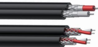
The RIG series cables are very high-quality signal cables for indoor fixed or mobile applications. They have a PVC jacket and are very easy to handle. The inner conductors are fitted with a durable tin plated copper shielding and an extra Aluminium mylar foil (RIG48 only). This gives an excellent protection against interference of all kinds, such as electromagnetic fields produced by dimmers, electric motors or power cables.
