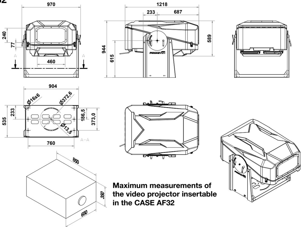
Maximum measurements of the video projector insertable in the CASE AF32
