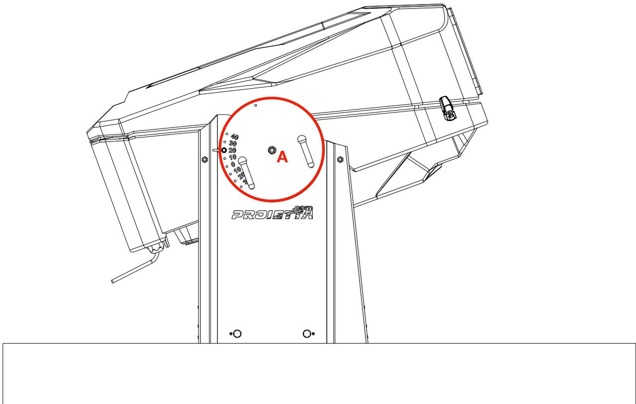
**WARNING:** Never unscrew the bolt (A) shown in the figure because it keeps the case assembled to the support bracket.
