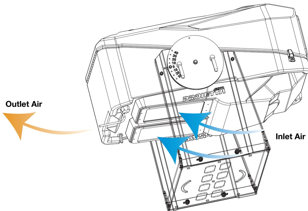
The air enters in the case at outdoor ambient temperature ( $T_{\text{INLET AIR}}$ ) from the filter-equipped air intakes located at the bottom of the case (there is only one air intake for the AF6 model).
