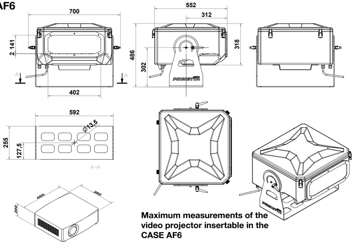
Maximum measurements of the video projector insertable in the CASE AF6
