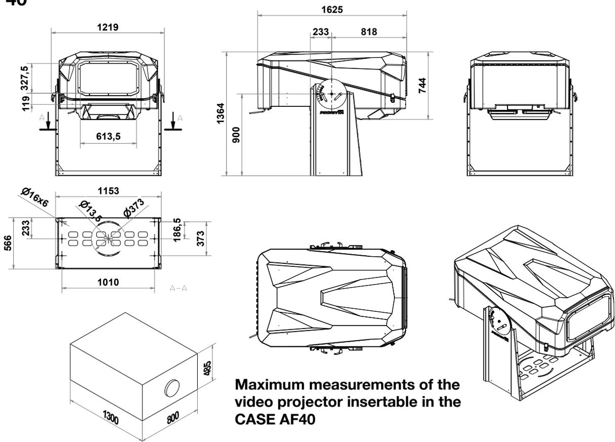
**Maximum measurements of the video projector insertable in the CASE AF40**
