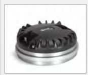
A new high performance 3.0 inch diaphragm compression driver with a 1.4 inch exit throat deliver perfectly natural midrange and high frequency. The diaphragm is precision formed from pure titanium, the suspension is based on a vented and damped design in order to provide very low distortion.
