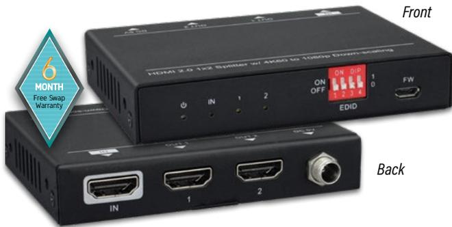
VLHDMISPIX2 is an ultra slim 1x2 4K@60Hz HDMI splitter that support different output resolution, like down scale to 1080P on one output. Built-in equalizer for signal enhancement, 18Gbps high bandwidth.
