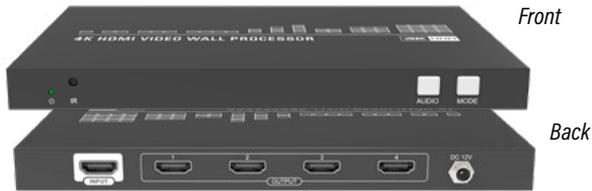
This Video Wall Processor has 1 HDMI input and 4 HDMI outputs. HDMI input supports resolutions up to 4Kx2K@60Hz 4:4:4 and output resolution is fixed to be 1920x1080p@60Hz. It supports 9 video wall modes, which can be selected via front panel button and IR remote.
