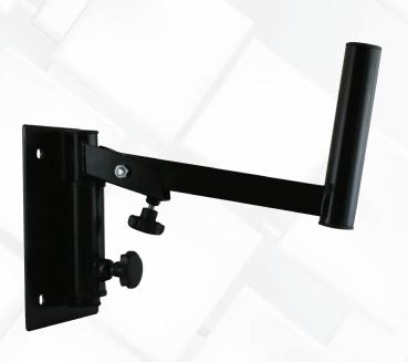
The SWB40 is a heavy duty wall mount bracket for loads up to 40 kg. It is slewable for 180° and tiltable from 90° to 110° downwards. The complete system is from black powder coated 2 mm steel.
