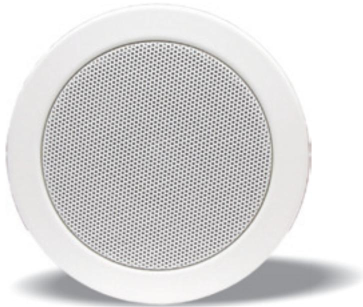
Modern and very compact built-in speaker provided with a 3" woofer. This loudspeaker has a "halogen-spotlight" size, what makes it ideal to integrate into each interior. The loudspeaker comes with a high quality 100 Volt transformer, 6 watt with several power tapings. The housing is made of metal. The loudspeaker itself is made of polypropylen, what makes it moisture-proof. The loudspeaker is easy to install, due to its simple, quick mounting system (2 spring-clamps)
