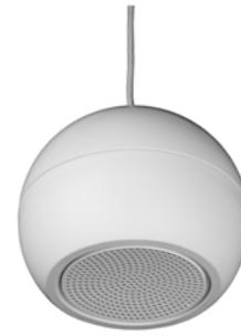
The EN-SPH5T16-W is a compact 5.25" sphere loudspeaker with ABS housing (UI94 HB) (RAL 9010 equivalent), equipped with a high efficiency full range speaker and a multi tap 100 volt transformer, all certified according EN 54-24.
