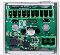
The AUDAC CP43/45ARP are wall junction boxes containing a repeater for extending the range of a digital audio signal transmitted over simple UTP CAT6 Cabling.
