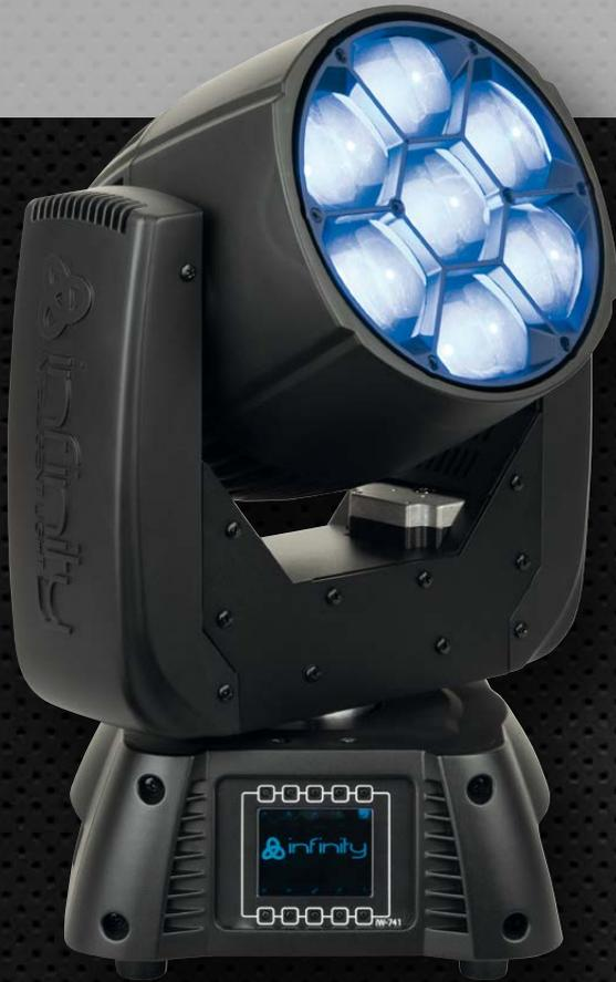
The Infinity iW-741 is a compact power-pack which is equipped with 7 RGBW 40W Osram LEDs. Especially selected motors provide ultrafast and precise movements. In combination with motorized zoom a razor sharp 3,6° beam can be produced which changes into a 60° wash effect through various available controlling protocols. The seven O-Star LEDs produce very bright and saturated colours and by changing the PWM through DMX the iW-741 is very well suited for theatre or television applications.
