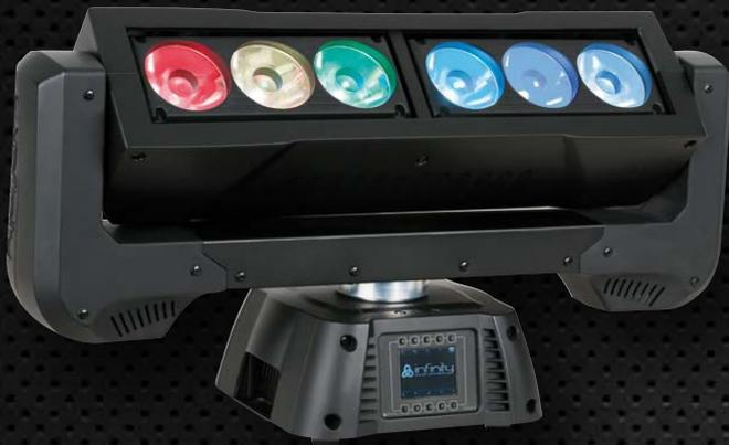
The Infinity® iFX-615 is a moving batten with 2 individual moving sections; continuous rotation on both X- and Y-axis, and 2 separate LED sections (3 LEDs each) with a movement of 15° in both directions.
