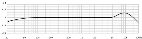
measured in free-field conditions (IEC 60268-6), tolerance  $\pm 2$  dB
