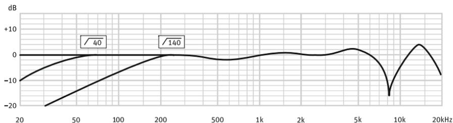
measured in free-field conditions (IEC 60268-4), tolerance ±2 dB
