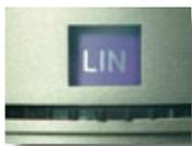
A steep high-pass filter in the LIN position prevents the output transformer of the microphone from being overloaded due to undesired subsonic frequencies.
