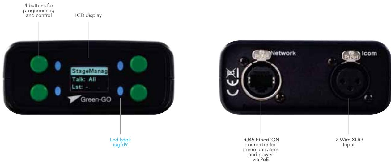
The 2W Slim Audio Interface links 2-wire analogue intercom systems into the Green-GO digital Ethernet network. The 3-pin XLR port will connect to the partyline system. The port can be configured through the setup menu. One of the channels on the partyline system then becomes a group on the Green-GO system.
