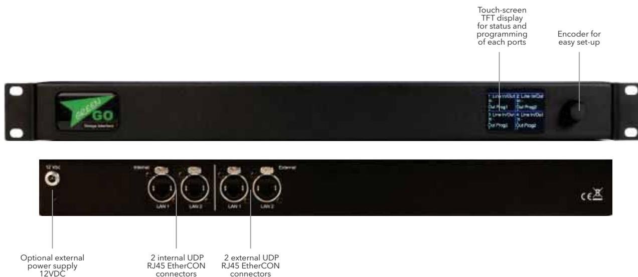
The Green-GO BridgeX provides (4) UDP network ports, intended to connect remote locations to a Green-GO network. This can be done in two separate modes; 'Bridge' mode or 'Remote User' mode. In both modes, the Green-GO BridgeX can support four connections.
