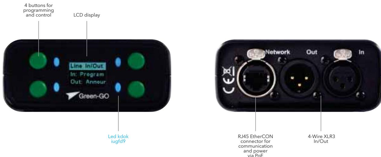
The 4W Slim Audio Interface links any 4-wire analogue intercom system into the Green-GO digital Ethernet network. This audio in/out interface connects either to an existing matrix or other analogue interfacing products. This allows an audio signal to be injected into the Green-GO network and transmitted to any other location on the same Ethernet network. When use as a matrix style intercom system, one channel of the matrix system can be used as a group on the Green-GO systems
