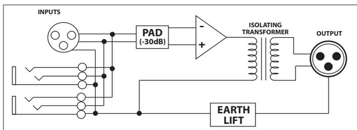
The DN100 is an active DI box providing transformer isolation impedance matching and attenuation into a low impedance active balanced input.
