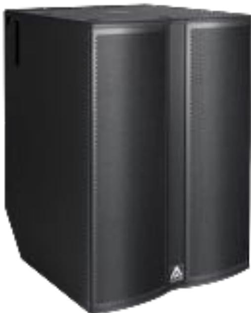
*The combination of two 18-inch woofers with 4-inch long excursion voice coil in a highly reinforced cabinet, with 2500 W amplification, DSP and ergonomic design, makes the N218W the right choice for high demanding applications.*
