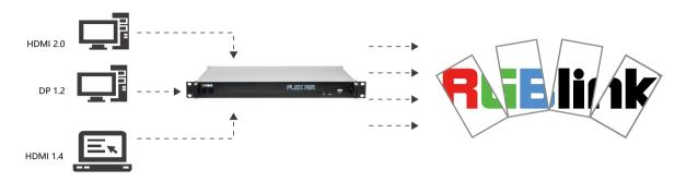
Each of the four outputs may be configured individually with rotation in 1 degree positioning. Video layered and mapped across the output displays.
