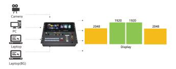
${\it Example: Multiple\ AUX\ outputs\ with\ separate\ scale\ configuration}$
