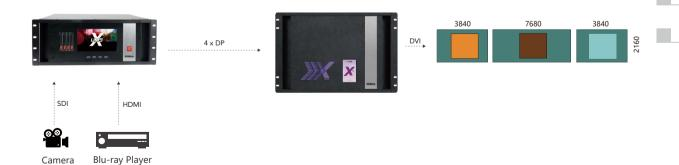
Example: UMS4 with SDI and HDMI capture cards installed. Media player software outputs content including the SDI and HDMI inputs as 4K DP outputs, these connected to an X7 video processor, which in turn allows a sources to be used as a scaled background and the others as a scaled foreground layers/windows.
