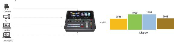
Example: Scaled output to each AUX output.
