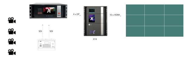
Example: UMS4 taking in video feeds from a production switcher, applying graphics then outputting to a video processor which splices and scales the video across an in studio video wall.
