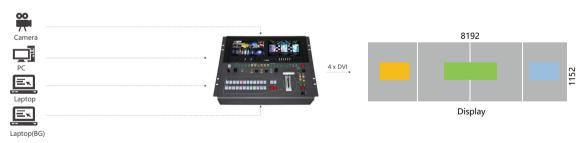
Example: Single PIPs on each of two displays as well as a PIP split across the two AUX outputs over a background
