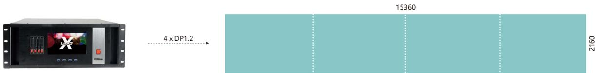
Example: UMS4 with media server software and content output directly to 4K displays with output arrangement via Windows/software
