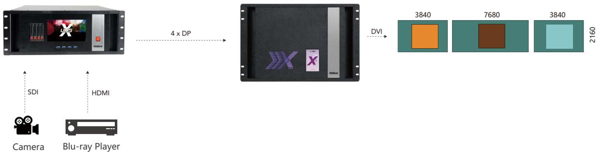
Example: UMS4 with SDI and HDMI capture cards installed. Media player software outputs content including the SDI and HDMI inputs as 4K DP outputs, these connected to an X7 video processor, which in turn allows a sources to be used as a scaled background and the others as a scaled foreground layers/windows.
