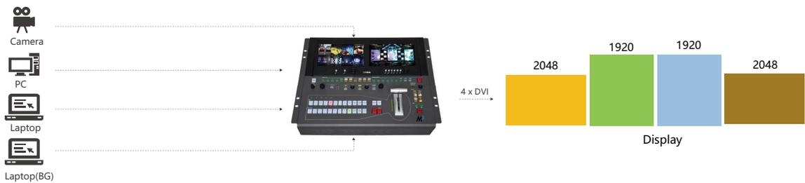
Example: Scaled output to each AUX output.
