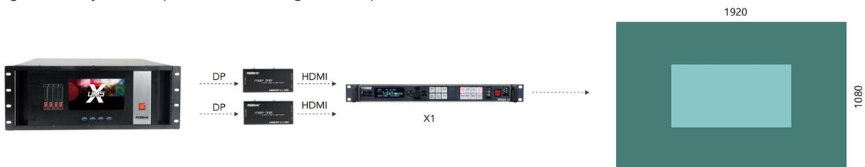
Example: UMS4 with media player software and on board content with two 2K outputs connected to an X1 video processor, which in turn allows 1 source to be used as a background and the other as a scaled foreground PIP.
