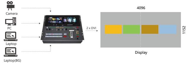
Example: two scaled video layers on each HDMI output
