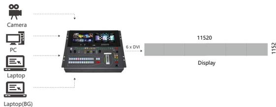
Example: 12K x 1K spliced display using six outputs
