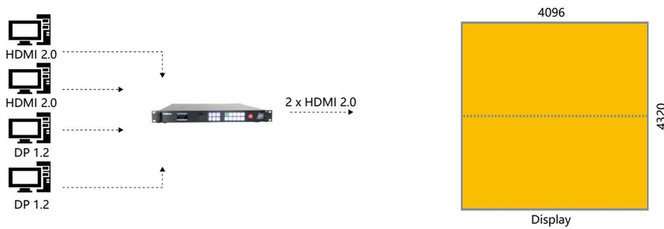
Example: 4K input scaled across 4K x 4K display area using two outputs, forming a seamless portrait display of
