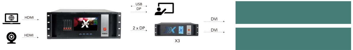
Example: UMS4 with collaboration software taking in laptop and camera sources, then outputting to touch screen display with side LED displays providing an extended canvas or duplication
