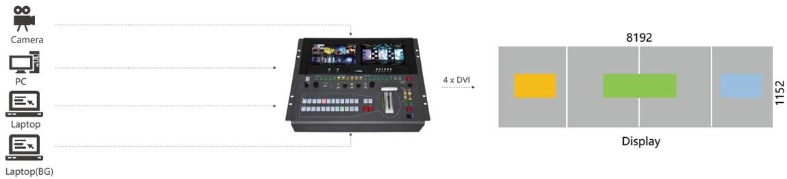
Example: Single PIPs on each of two displays as well as a PIP split across the two AUX outputs over a background
