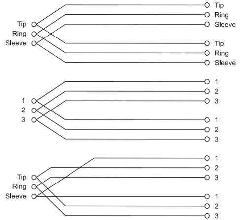
**Headphone Separator** Note: for every doubling of headphones the load impedance is halved. Do not go below 150 Ohms.
