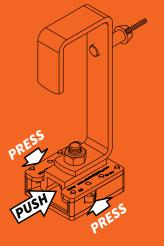
Pull the hook backwards into the housing, press both locks and slide the hook outwards.
