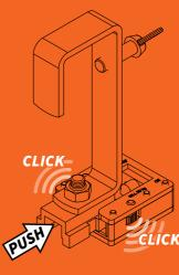
Push the clamp part against the spring block inside the Luminaire part until both locking switches are activated.
