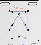
40 truss  $\triangle$  and  $\square$ (centre-to-centre distance 329 mm)
