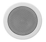
The EN-CM5T6 is a 5.25" built-in ceiling speaker made of powder coated steel (RAL 9010 equivalent), equipped with a high efficiency full range speaker and a multi tap 100 volt transformer, all certified according EN 54-24.
