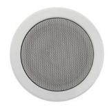
The EN-CM6T6 is a 6.5" built-in ceiling speaker made of powder coated steel (RAL 9010 equivalent), equipped with a high efficiency full range speaker and a multi tap 100 volt transformer, all certified according EN 54-24. The unit is equipped with a ceramic speaker line connector block, thermal fuse and a metal fire dome.
