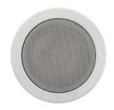
The EN-CMX6T10 is a built-in 2-way ceiling speaker made of powder coated steel (RAL 9010 equivalent), equipped with a high class 2-way speaker and a multi tap 100 volt transformer, all certified according EN 54-24, offering a detailed and powerful sound for demanding applications.
