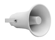
The EN-H15-G is a powerful horn speaker made of UV and impact resistant ABS (RAL 7035 equivalent), (UL94V0), equipped with a compression driver and a multi tap 100 volt transformer, all certified according EN 54-24. IP66 makes it the ideal choice for industrial applications.
