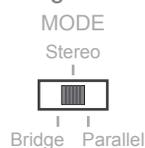
It is default configured in stereo mode (center position) whereby each amplifier channel is fed with an individual input signal. In bridge mode (left position), the power of both channels is merged for delivering double power to a single load. In parallel mode (right position), the input is linked, feeding the identical signal to both channels.
