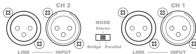
An operation mode switch allows switching the channels between stereo, bridge and parallel mode.
