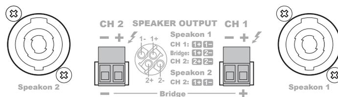
The 'Speakon 1' output connector carries signals for both both channels, allowing connection for both channels through a single 4-core cable or bridge mode connections.
