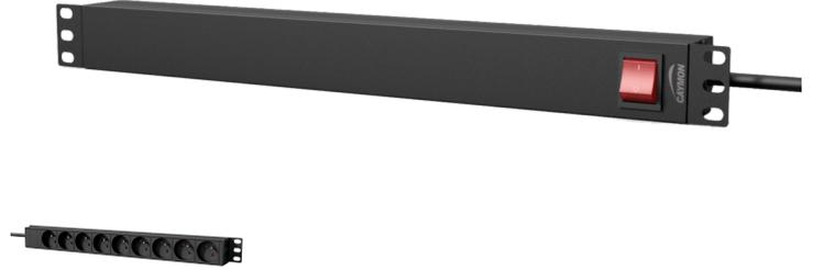
The PSR1x9Fx are 19" power distribution units, compliant to the ANSI/EIA RS-310D, DIN41491 and IEC60297 standards. They come in three different models, without a switch (PSR109F), with an illuminated switch on the socket side (PSR109FS) or with an illuminated switch on opposite of socket side (PSR119FS). The construction is made using black powder coated aluminum fitted with steel 19" mounting ears on each side.
