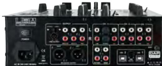
**CORE MIX-4 USB****D2304** 4 Channel DJ mixer with USB interface
