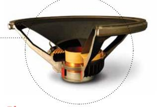
BI Expressed in Tesla meters is a measurement of the motor strength of a speaker. This is created by the product of the magnetic field strength times the length of wire in the field. If you were to take a given mass, that when placed on the cone of a speaker would move the cone downward from its home position, then measure the current in amperes required to move the cone back to home position, you can calculate Bl. The formula is Ma in grams divided the current in amperes
