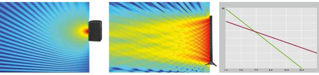
The sophisticated BEM simulation, applied here at 3 kHz, clearly shows that line arrays (right) disperse sound far better than conventional systems (left). Red and yellow hues signify high sound pressure levels; dark blue indicates low levels.
