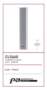
Power rating: 60 W RMS Available power: 60 W / 30 W at 100 V Speaker: 6 x 2.5 inches Frequency response: 250 Hz -15 KHz Sensitivity (1 W @ 1 m): 96 dB Aluminium body and grill, Ingress protection: IP44 (weather-resistant) Dimensions: 104 x 73 x 550 mm Weight: 2.6 kg
