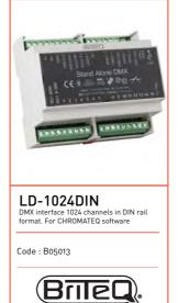
Interface in DIN rail format 1024 DMX channels Compatible with "Chromateq Led Player" and "Chromateg Pro DMX" software. (supplied) Internal 4MB memory for storing programs. Internal memory for max. 255 scenes Activation by external contacts or optional remote control Calendar function Splitter mode 2x512 Merger mode Chaining in Master/Slave possible Operating system: Windows & MAC OSX & Linux DMX inputs and outputs on connectors. Power supply: By mini USB 5V or Art-Net Universe available: 2
