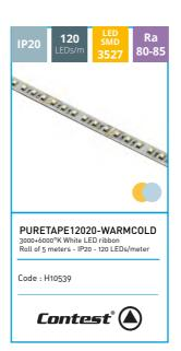
Two-tone adhesive ribbon of 600 warm and cold white LEDs for 5m Width: 10 mm Colour temperature: 3500K/6500K Luminosity: 1264 lumens/m Power required: 19.2 W/m (96W for 5m) Voltage required: 24V (+ and -) Cuttable every 5.3cm (6 LEDs) IP20: no protection no sealing
