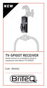
This special adapter makes it possible to easily connect a standard clamp to equipment with 28mm TV-SPIGOT Perfect to fix our BT-THEATRE YOKE (code: B06021) to a standard clamp like our: FAST CLAMP V2 (code: B02684) ULTRA CLAMP (code: B06600) Metal: AL6061-T6 SWL: 100kg Color: black
