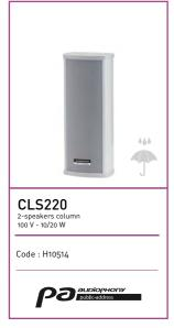
Power rating: 20 W RMS Available power: 20 W / 10 W at 100 V Speaker: 2 x 2.5 inches Frequency response: 250 Hz -15 KHz Sensitivity (1 W (0 1 m): 94 dB Aluminium body and grill, Ingress protection: IP44 (weather-resistant) Dimensions: 104 x 73 x 262 mm Weight: 1.4 kg
