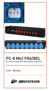
Outputs on 8 IP54 outlets Standard French plugs 8 bipolar switches 6.3 amp fuse for each channel the total charge cannot exceed 15 amps (3300 W) Rackable 19 inches / 2U Dimensions: 483 x 80 x 97 mm Power supply: 230V - 50 Hz Weight: 2 kg
