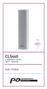
Power rating: 40 W RMS Available power: 40 W / 20 W at 100 V Speaker: 4 x 2.5 inches Frequency response: 250 Hz -15 KHz Sensitivity (1 W @ 1 m): 95 dB Aluminium body and grill, Ingress protection: IP44 (weather-resistant) Dimensions: 104 x 73 x 402 mm Weight: 194 kq
