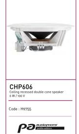
Power rating: 6 W RMS Available power: 6 W / 3 W at 100 V Speaker: double cone 6.5 inches Frequency response: 110 Hz – 13 kHz Sensitivity (1 W @ 1 m): 90 dB External dimensions (diameter and depth): 230 x 90 mm Drilling diameter: 200 mm Net weight: 0.9 kg
