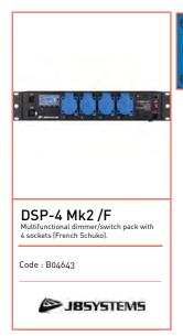
Power rating: 8 A (1850 W) per channel / 15 A max. resistive/inductive Protection of each channel by fuse Independent addressing of each channel LED display with drop-down menu Power supply: 240V - 50Hz single phase 4 16A French plug outputs on the front DMX XLR 3 input and output Dimensions: 482 x 100 x 88 Weight: 2.9 kg
