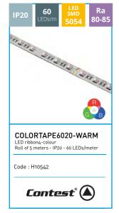
Ribbon of 300 4-colour RGBW LEDs for 5m Width: 12 mm Luminosity: 879 lumens/m Power required: 19.2W/m (96W for 5m) Voltage required: 24V (+ and -) Cuttable every 10 cm (6 LEDs) IP20: no protection no sealing
