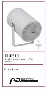
Power rating: 10 W RMS Available power:  $10\ W/5\ W/2.5\ W\ at 100\ V$  Frequency response: 150 Hz – 14 kHz Speaker: 5 inch Sensitivity (1 W (8 1 m): 90 dB White aluminium body, lngress protection: IP55 (weather-resistant) Dimensions (0 x D): 138 x 205 mm Weight: 2.1 kg
