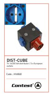
Cube format distributor 2 M10inserts Tetra CEE 16A input plug 3 16A standard German plugs (1 outlet per phase) Dimensions: 160 x 136 x 102 mm Weight: 0.86 Kg
