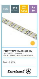
Double monochrome adhesive ribbon of 720 warm white LEDs for 5m Width: 20 mm Colour temperature: 3000°K Luminosity: 2452 lumens/m Power required: 47.5W/m (238W for 5m) Voltage required: 24V (+ and -) Cuttable every 8.4 cm (12 LEDs IP20: no protection no sealing
