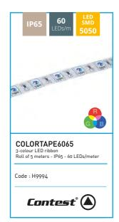
Trichromatic adhesive ribbon of 300 RGB LEDs for 5m Width: 11 mm Luminosity: 510 lumens/m Power required: 14.4W/m (72W for 5m) Voltage required: 24V (+ and -) Cuttable every 10 cm (6 LEDs) IP65: Upper molded silicone dome
