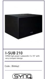
Power rating: 500 W RMS Frequency response: 50Hz -200Hz SPL 1w/1m : 98 dB Nominal impedance:8  $\Omega$  Woofer: 2x10" Connectors: 2 x speakon Dimensions: 600 x 350 x 410 mm Net weight: 26 kg
