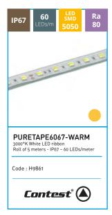
Monochrome adhesive ribbon of 300 warm white LEDs for 5m Width: 12,5 mm Colour temperature: 3000°K Luminosity: 1080 lumens/m Power required: 14,4W/m (72W for 5m) Voltage required: 24V (+ and -) Cuttable every 10 cm (6LEDs) IP67: Full silicone sheath
