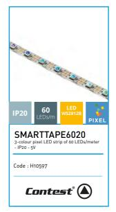
3-colour adhesive ribbon of 300 RGB LEDs for 5m pixel version Width: 10 mm Power required: 14.4W/m (72W for 5m) Voltage required: 5V DC Cuttable every 1.6 cm (1 LED) IP20: no protection no sealing
