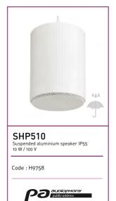
Power rating: 10 W RMS Available power: 10~W/5~W/2.5~W~at~100~V Frequency response: 150~Hz – 15~kHz Speaker: 5 inch Sensitivity (1 W (0 1 m): 90 dB White aluminium body, Ingress protection: IP55 (weather-resistant) Dimensions (0 x D): 138 x 205 mm Weight: 2.2 kg
