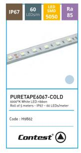
Monochrome adhesive ribbon of 300 Colour temperature: 6000° K Width:12,5 mm Luminosity: 1170 lumens/m Power required: 14.4W/m (72W for 5m) Voltage required: 24V (+ and -) Cuttable every 10 cm (6LEDs) IP67: Full silicone sheath
