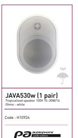
Power outputs: 15 / 30 W Voltage : 100 V 16 Ohms Components : 5" + 1" Sensitivity (1W/1m): 88 dB, +/-3dB Frequency response : 60 - 20 000 Hz Material : Plastic enclosure and aluminium grille Holding : Wallmount bracket
