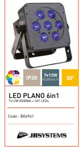
7x12W six-colour RGBWA + UV LEDs Beam opening: 30° Infrared remote control Ready for a DMX wireless connection with the WTR-DMX option Digital display with drop-down menu Input and output on IEC plugs Modes of operation: Standalone, Master/slave mode, DMX mode, usable with LEDCON-XL controller DMX input and output Power consumption: 50 W Power supply: AC 100/240V - 50/60Hz
