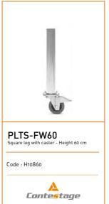
Material: Aluminium Thickness: 3 mm Section: 60 x 60 mm Wheel diameter: 100 mm Weight: 2.06 Kg
