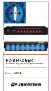
Outputs on 8 IP54 outlets Standard German plugs 8 bipolar switches 6.3 amp fuse for each channel the total charge cannot exceed 15 amps (3300 W) Rackable 19 inches / 2U Dimensions: 483 x 80 x 97 mm Power supply: 230V - 50 Hz Weight: 2 kg
