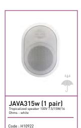
Power outputs: 7.5 / 15 W Voltage : 100 V 16 Ohms Components : 3" + 1" Sensitivity (1W/1m): 90 dB, +/-3dB Frequency response : 90 - 20 000 Hz Material : Plastic enclosure and aluminium grille
