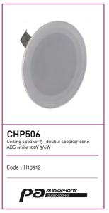
Power outputs: 3 / 6 W Voltage: 100 V Components 5" loud-speaker Sensitivity (1W/1m): 93 dB, +/-3dB Frequency response: 100-15 000 Hz Material: Metallic grille and plastic enclosure Holding: 2 string grip Connectors: 3 contacts connector Drill hole diameter: 145mm Dimensions: 160(diam) x 54 (H) mm Weight: 500 g
