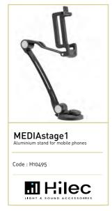
For 3.5 to 5.5 inch phones Material: Aluminium Dimensions (WXHxD): 38 x 381 x 25 mm Folded dimensions (WXHxD): 38 x 168 x 25 mm Arm length (unfolded): 238 mm Stand depth: 17.5 mm Stand height: 57 to 89 mm Weight: 130 grams
