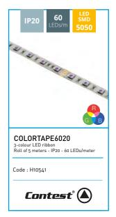
Trichromatic adhesive ribbon of 300 RGB LEDs for 5m Width: 10 mm Luminosity: 560 lumens/m Power required: 14.4W/m [72W for 5m] Voltage required: 24V [+ and -] Cuttable every 10 cm [6 LEDs] IP20: no protection no sealing
