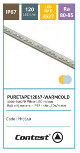
Two-tone adhesive ribbon of 600 warm and cold white LEDs for 5m Width: 12,5 mm Colour temperature: 3500K/6500K Luminosity: 1264 lumens/m Power required: 19.2 W/m (96W for 5m) Voltage required: 24V (+ and -) Cuttable every 5.3cm (6 LEDs) IP67: Full silicone sheath
