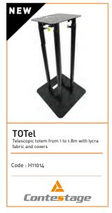
Minimum height: 1 m Maximum height: 1.80 m Lower base: 50 x 50 cm Upper base: 30 x 35 cm Diameter of the base tubes: 43 mm Diameter of telescopic tubes: 35 mm 2 safety pins 2 adjustment wheels Cable passage 11 x 4 cm Supplied with 35 mm x 125 mm speaker top mount Supplied with white Lycra fabric Comes with a cover for the bases and a cover for the feet Material: Steel Finish: Black paint Weight: 18 Kg Maximum capacity: 30 Kg
