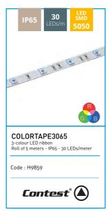
Trichromatic adhesive ribbon of 150 RGB LEDs for 5m Width: 10 mm Luminosity: 255 lumens/m Power required: 7.2W/m (36W pour 5m) Voltage required: 24V (+ and -) Cuttable every 16,8 cm (6 LEDs) IP65: Upper molded silicone dome
