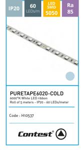
Monochrome adhesive ribbon of 300 cold white LEDs for 5m Width: 10 mm Colour temperature: 6000°K Luminosity: 1190 lumens/m Power required: 14.4W/m [72W for 5m] Voltage required: 24V [+ and -] Cuttable every 10 cm [6LEDs] IP20: no protection no sealing
