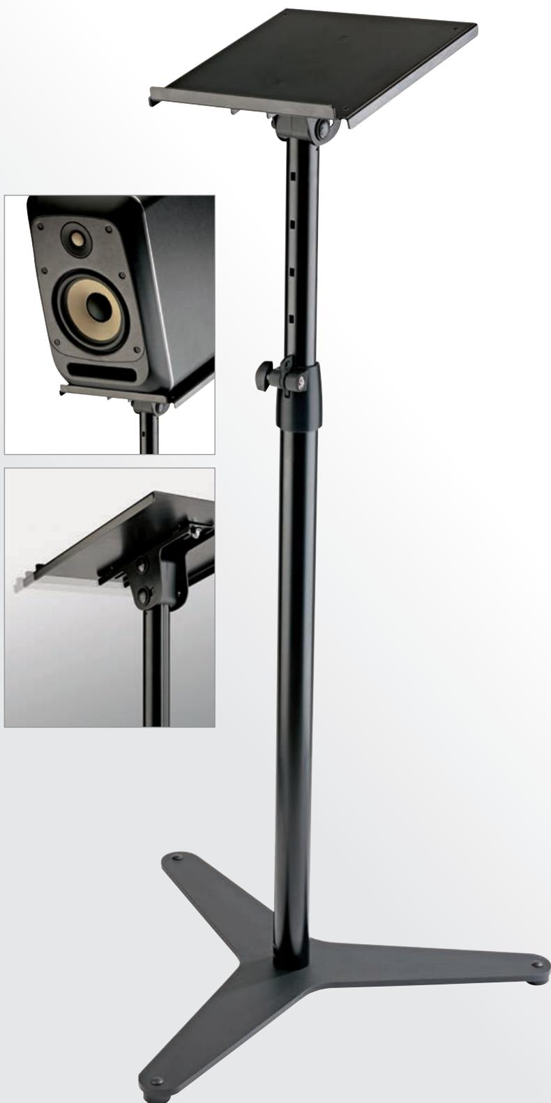
The modern studio monitor stand with a tiltable tray and a metal tripod base provides for stability and functionality. The three felt pads ensure noise filtration. The adjustments for the monitor tray include a 12.5° angle and 45 mm in depth. The stop angle of the tray provides additional safety. The height is adjusted by a clamping lever and ranges from 800 to 1300 mm. The gradual height adjustment to the desired positions takes place in 50 mm intervals.
