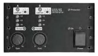
Detachable front panel gives access to a limiter threshold adjust. (LIMITER)
