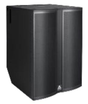
The combination of two 18-inch woofers with 4-inch long excursion voice coil in a highly reinforced cabinet, with 2500 W amplification, DSP and ergonomic design, makes the N218W the right choice for high demanding applications.
