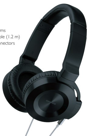
Wide-range 40 mm dynamic driver, bass-reflex enclosure, earpad, aluminum driver housing, and hanger arm
