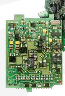
The amp's QuantaPulse EVO brain, in the line of our classic function controllers, watches over more parameters and is far more compact as a result of SMD technology. Communication between the power supply and the audio amplifier is absolute.
