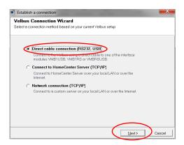
The software will automatically choose the port on which the Velbus USB module is connected. Click Finish to automatically establish a connection and start configuring your devices.
