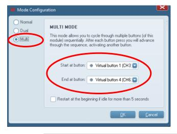
If the option Restart at the beginning if idle for more than 5 seconds is selected, after 5 seconds of inactivity, pressing the button will activate the first button in the series. If not, the module will remember the last channel that has been activated and continue from there.
