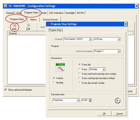
In the Program Step Settings dialog, the details of the program step can be configured. When all fields have been set as needed, click on OK to to add the program step.
