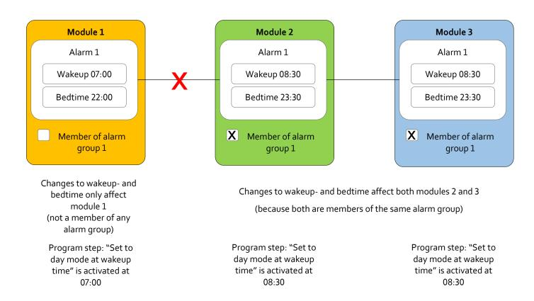
Eg. the temperature sensor of multiple modules needs to be set to day mode in the morning. In each of the modules a program step "set to day mode at wakeup time" is created. All modules are made members of the same alarm group. If the wakeup time needs to be adjusted later on, it suffices to change it in one module. The other modules will automatically copy it.
