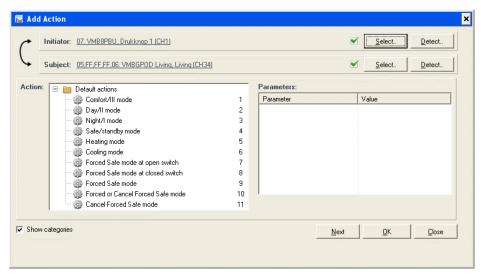
Available actions are switching to day/night/safe/comfort mode, to heating or cooling mode, and so on.
