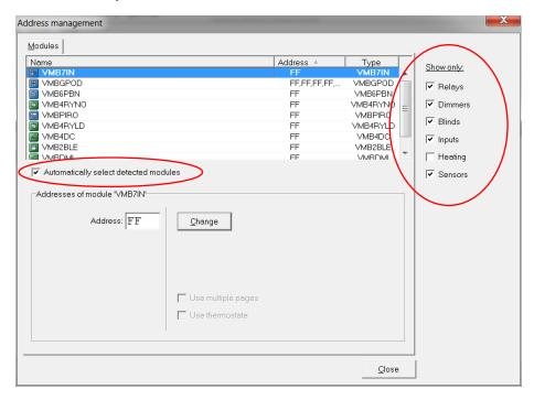
If you now physically press a button on a module, the module will be automatically selected in VelbusLink for you to change its address. (As soon as a module has been detected, the Automatically select detected modules option will be unticked in order to avoid confusion if someone else would accidentally push a button).
