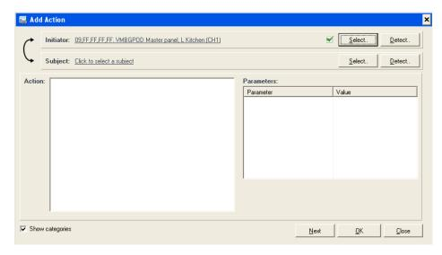
As before, the Add action window will appear, and the input selection will be pre-populated with the button selected here. Note the double arrow to the left of "initiator" and "subject": clicking on the arrow will switch the selected channels around.
