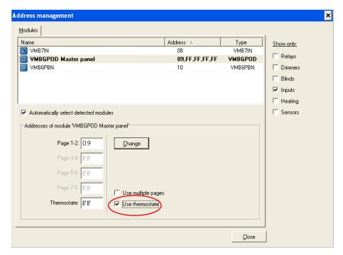
Check the Use thermostat checkbox. The input field for the thermostat will become active. Fill in a free address between 01 and FE and press Enter or click on the Change button. Do the same for other modules as necessary. Then press Close.
