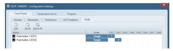
Double-click the button that needs to function in dual mode (in our example Push button 1 (CH1)). The dialog Mode configuration appears (see screenshot below). Select Dual on the top left. Then select to the right the first channel of the series (in our example Virtual 1 (CH3) and the last (in our example Virtual 4 (CH6)). This way, at each button press on Push button 1 (CH1), virtual button 1 (CH3), then 3 (CH5) and 4 (CH6) will be activated.
