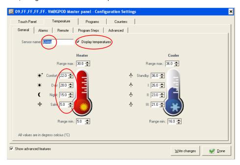
In the VMBGPOD configuration settings, do the same as above for the VMBGP2, and also check the Display temperatures checkbox. This makes the thermostat page accessible on the OLED display of the VMBGPOD.
