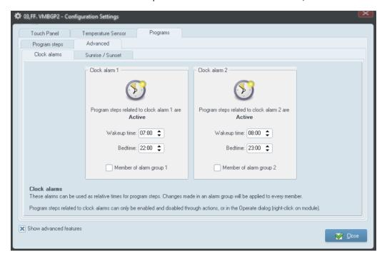
Wakeup- and bedtimes can be seen as variables, whose value can be set in the tab Programs > Clock alarms of VelbusLink, or on the oled screen of a VMBGPOD glass control module. The scope of this variable is initially limited to the module. But wakeup- and bedtimes can be made member of alarm groups. In that case, when the value is changed for one member of the group, all other members of the group will copy this value.
