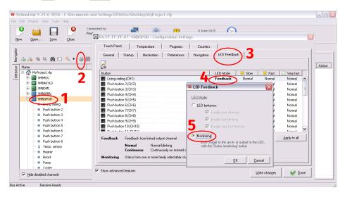
Step 2 is defining which output channel has to be monitored. Create the following action (see also "Actions" p.13):
