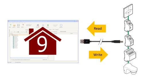
In VelbusLink reading means: copying the physical module's contents to the PC, overwriting the VelbusLink project. Writing means: copying the VelbusLink project from your PC to the memory maps of the modules, overwriting the modules.
