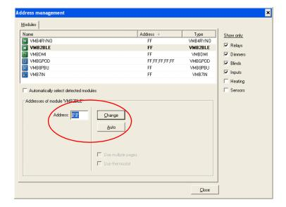
Addresses of selected modules are changed by entering a new value (01 to FE hexadecimally, or 0-254 decimally) in the address field. You can also change the name of the module by clicking on it and entering a new name (see screenshot below).
