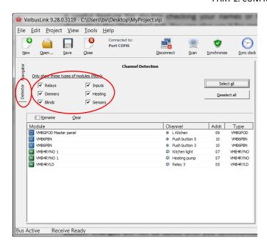
First, make sure the types of modules you want to be detected (relays, dimmers, inputs, ...) are checked in the top section of the detector window. Here you can filter out modules by unchecking the groups they belong to. This can be useful to ignore modules that periodically put data on the bus (like temperature or movement sensors) and that would otherwise appear without being activated by you.
