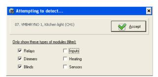
Pressing Accept will fill in this channel in the Add action dialog at the appropriate place. You can then select the type of action you want to happen. (Remember to modify any parameters in the right hand pane if necessary.)
