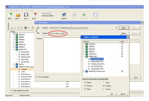
Each module's channels are only shown after the module has been expanded (by clicking on the + sign to the left of it). If you can't find the module you're looking for, make sure its type is checked in the filter at the bottom of the Select a channel dialog.
