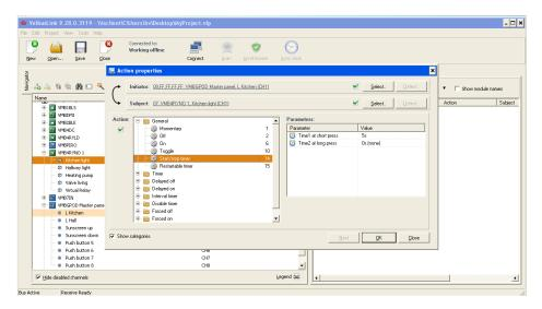
All that remains to do to complete the configuration of the action is to define the type of action that you want to happen when this button is pressed. If necessary, the action parameters (for instance a delay time) can be specified in the right hand panel.
