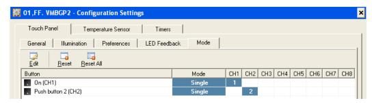
Double click the button that needs to be set to dual mode (in our example channel 1 "On"). The Mode configuration dialog pops up. Select Dual in the upper left corner. Then select next to Long press button which (virtual) button needs to be activated on long press. In our example, we select "Off" (channel 8).
