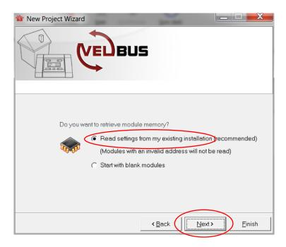
We recommend Read settings from my existing installation, as this is the only way to be sure that your project configuration in VelbusLink matches the actual configuration in the physical modules.
