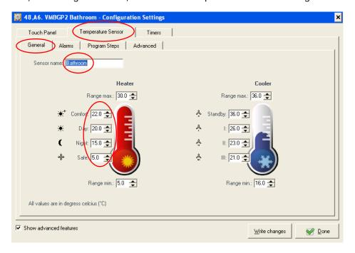
Edit the settings in the tab Temperature > General. Change the sensor name (we chose "Bathroom"), and set the desired target temperatures for each heating mode. The sensor name chosen here will also appear on the VMBGPOD display when we configure this later on. Click on Done.
